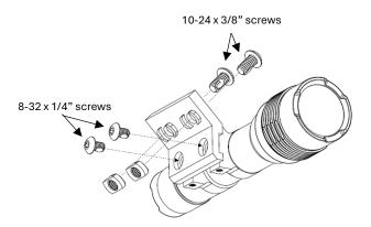
To connect the ProTac<sup>®</sup> Rail Mount and M-LOK<sup>®</sup> mount to the rail, rotate the M-LOK<sup>®</sup> T-nuts to the install/uninstall position. Position this assembly in the desired rail location. Tighten the 10-24x3/8" screws using the 1/8" hex wrench to lock the T-nut.
