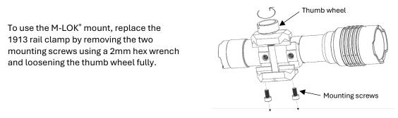
Align the M-LOK<sup>®</sup> mount holes with the ProTac<sup>®</sup> Rail Mount holes and use the 3/32" hex wrench to tighten the 8-32x1/4" screws.
