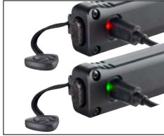
Charge indication LED Red: Charging Green: Charged
