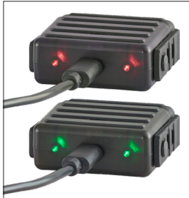
Charge status indicator lights RED CHARGING | GREEN CHARGED
