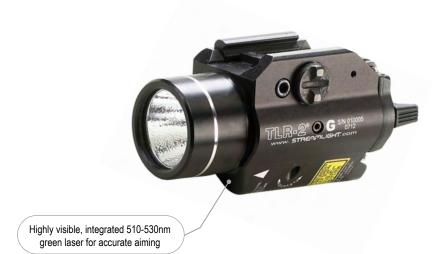
Material/Lens 6000 Series machined aircraft aluminum with black anodized finish. High-impact, chemical resistant engineering polymer laser housing. High temperature, shock-mounted, impact-resistant BOROFLOAT® glass lens; gasket sealed.
