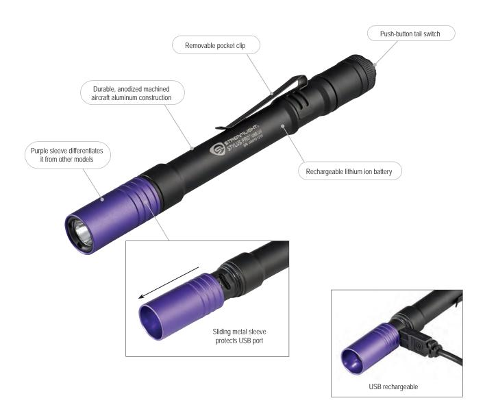
400 nanometer UV LED: 250 mW measured system output; runs 2.5 hours Fully regulated output for consistent UV performance over the battery life
